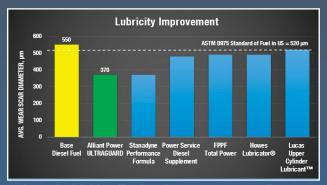
Increasing lubricity will reduce the average wear scar diameter of base fuel resulting in minimized friction and wear of critical fuel system components.
